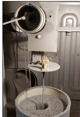
Dust tolerant connectors and mechanisms being tested in TVAC with various lunar simulants
