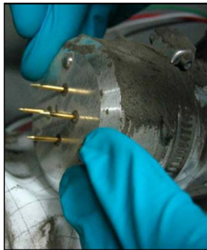
Dust tolerant connectors and mechanisms being tested in TVAC with various lunar simulants
